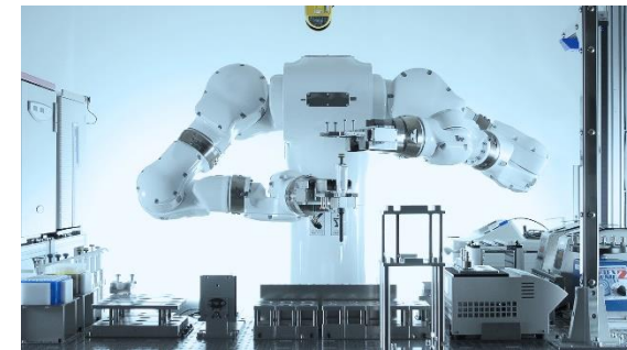
"Maholo", a dual-arm robot designed and marketed for biomedical applications
