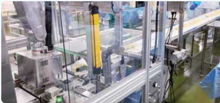
Operation of the lid-closing robot
